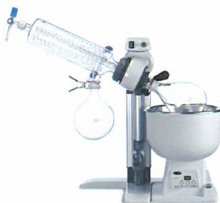
Fig. 1-21 Example of experimental equipment for removal of organic solvent
