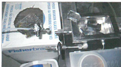
Fig. 3-30 Rupturing of the chamber due to excessive supply of gas
