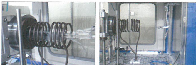
Fig. 3-29 Inside the MOCVD reactor prior to and following gas explosion
