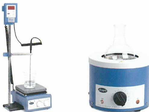
Fig. 1-23 Examples of high temperature device(heated agitator and heating mantle)
