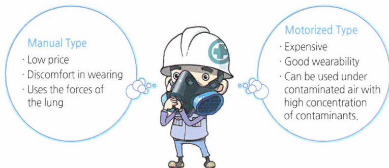
Fig. 1-5 Advantages and disadvantages of manual type and motorized air purification type respiratory protection devices
