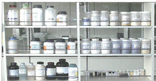
Fig. 3-2 Storage of chemical substances (for each characteristics and phases, and distinguish those that cannot be stored together)
