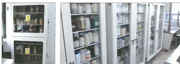
Fig. 3-3 Closed type ventilated reagent cabinet for hazardous reagents
